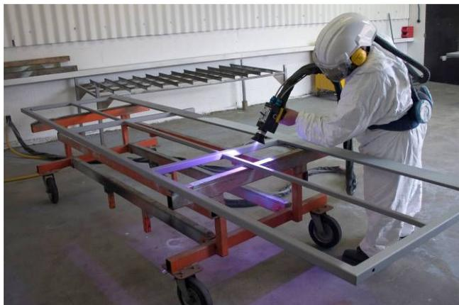
The operator has found it easy to use and is happy to work with the system. Herbert also purchased a 20m supplies package, which allows its operators to locate the spray unit outside the spray room and provides flexible access around the items they are spraying without having to stop to
