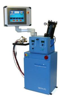
The thermal spray cell enables Vector Aerospace to apply a full range of coatings including, metallic bond coats, repair materials, ceramics and abradables. The cell primarily incorporates the Metallisation PS50M mass flow controlled Plasma system and the Metallisation 140/S250 Arcspray automatic system. The tilt and turn turntable provides an additional two axes to the six axis robotic manipulator, ensuring that all areas of the component are accessible for the coating.
