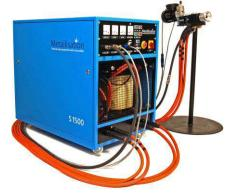
With huge demand for these towers and the large surface areas to be protected, it was immediately apparent that conventional manual thermal spray systems would not efficiently cope. It was also clear that standard automated systems would struggle to meet this demand. However, Metallisation's proven ARC528E-ACD/S1500 systems, operating at up to 1500A offered the ideal solution.
