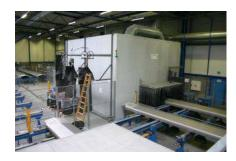
The fully automated metal spray facility is an acoustic booth containing two robots, one positioned above and one below each panel. One of the pistols has been modified from its standard configuration to enable better access. This ensures a high quality coating is applied to the underside of each panel. An electronically synchronised push/pull system is used under
