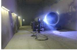
longest 36m tower section. The ability to have the power supply outside the dusty spraying area also improves reliability, efficiency and makes preventative maintenance a simpler and cleaner process.
