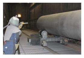
sprayed are grit blasted to standard SA3, while the areas that are painted, and not metal sprayed, are prepared to standard SA2.5. Mabey Bridge has a dedicated blast booth with programmable rotators, which provides a safe, clean and efficient area for the blasting process. During the QA/QC process, the profile and cleanliness of the blasted surfaces are checked and approved before metal spraying and painting can begin.
