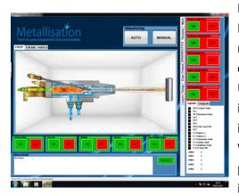
In order to optimise functionality and reliability the Met-PCC HVOF system control elements have been re-designed. Utilising the latest technology the operator interface now has an intuitive Graphical User Interface (GUI), which includes the option to integrate video images into the display. The interface operates on a familiar touchscreen Windows PC platform with Intel Dual Atom processor, which is ideal for operator usability, integration and communication.
