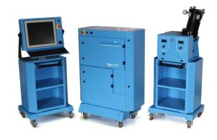
system and is available in two versions: The Met-PCC HVOF-L (liquid fuel), and the Met-PCC HVOF-G (gas fuel).
