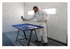
Fluorocarbon Surface Technologies applies both wet paint and powder based coatings in the booth, including ceramic based coatings for the pharmaceutical and food industries. There are plans in the near future to use the booth to produce dipped powder coatings with the introduction of a fluidised bed powder coating plant.
