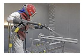
Fluorocarbon Surface Technologies blasts a variety of objects in the blast room, the largest item blasted so far is a 2.5m diameter vessel weighing in at approximately 1.5 tonnes. Due to the success, high performance and efficiency of the new blast room, Fluorocarbon is using it more frequently for the blasting of general items. The object being blasted in
