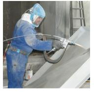
Metal spraying involves the projection of small molten particles onto a blast prepared surface. Upon contact, the particles flatten onto the surface, freeze and mechanically bond, firstly onto the blasted substrate and then onto each other, as the coating thickness is increased. To create the molten particles, a heat source, a spray material and an atomisation/projection method are required.
